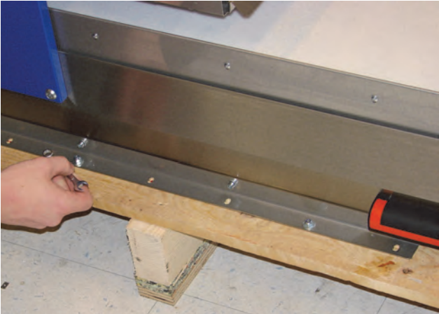
Figure 2-2. Shipping Screws on Mounting Rail
