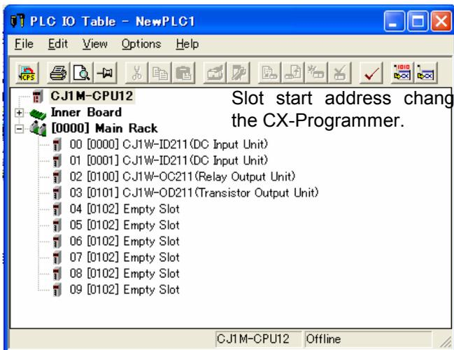
Slot start address changed on the CX-Programmer.
