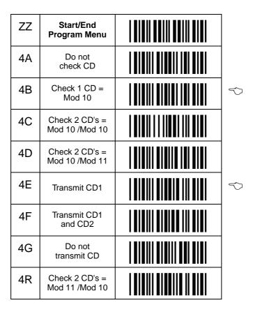
**MSI Plessey** is a variable length symbology with one or two optional check digit calculations CD1 and CD2 and non-printable start/stop characters. Supported characters include numeric digits 0 through 9.
