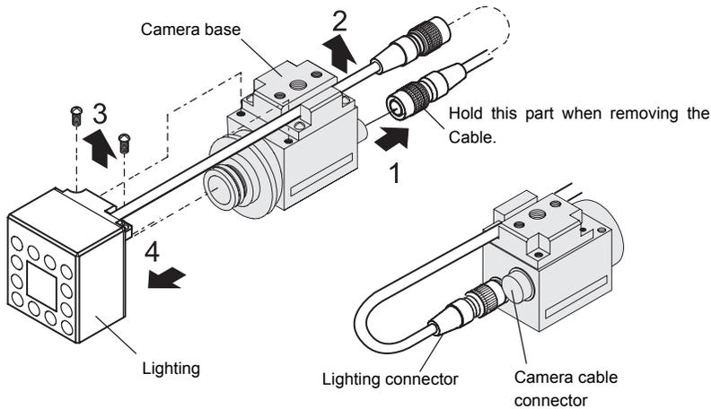
1. Disconnect the light cable from the light connector on the back of the Camera.
