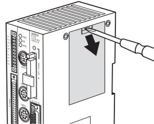
The battery is installed behind this cover.
