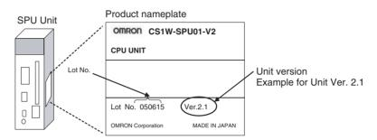
**Checking the Unit Version** from the SPU-Console from the SPU-Console Clicking the Unit Information Tab and displaying the System Information Tab Page. The unit version appears next to the model number in the *Product Information* Area. The unit version can be checked from the CX-Programmer (Ver. 4.0 or higher) by selecting **Unit Manufacturing Information**.
