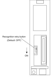
1,2,3... 1. Turn ON the recognition retry switch on the back of the SYSMAC SPU Unit.
