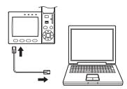
Use a commercially available LAN cable to connect the Controller to the PC.
