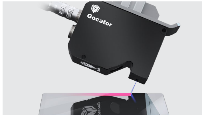
Gocator® 2512 scanning cell phone cover glass assembly
