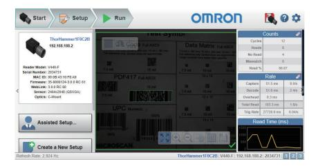
**5** Click on the **Setup** tab and set the *Cycle* to *Triggered*.
