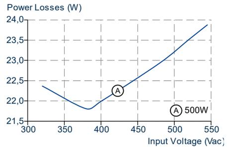
Fig. 9-4: Losses vs. input voltage at 24V, 500W, typ.
