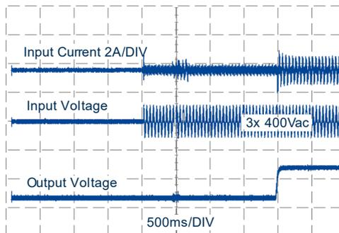
Fig. 5-1: Typical turn-on behavior at nominal load and 25°C ambient temperature
