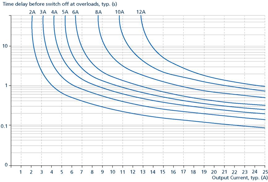
Fig. 6-1: Trip curve diagram for max 12A
