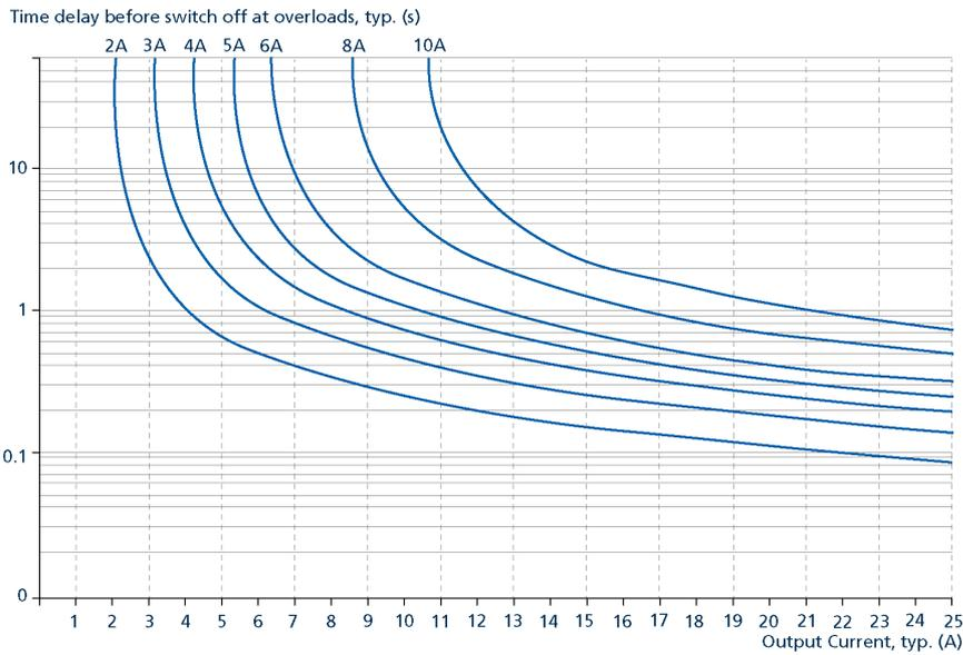
Fig. 6-2: Trip curve diagram for max 10A
